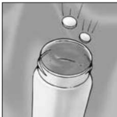
**2.** Drop two Dissolved Oxygen TesTabs® into the vial. Water will overflow when the tablets are added.
