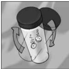
**4.** Mix by inverting the vial over and over until the tablets have dissolved. This will take about four minutes.
