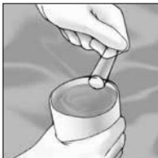
**1.** Submerge the small glass vial into the water sample. Carefully remove the vial from the water sample, keeping the vial full to the top.
