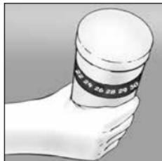
**2.** Remove the thermometer from the water and read the temperature (the number with the green background on the high-range thermometer). Record the number in degrees Celsius.
